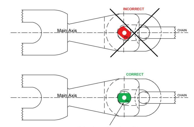
Flat surfaces of the pin must be connected parallel to the Main Axis
